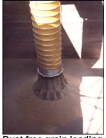
**Dust free grain loading** into barges.
