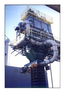
Model OV58 shown w/unique DCL dust collector integral w/ belt conveyor headchute.
