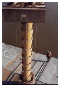
Heavy duty flex style spouts use inner cones to contain product flow enclosed by an outer sleeve for dust withdrawal. Inner cones are available in durable, lightweight urethane, carbon steel in hardnesses to 700 BHN, or in stainless steel.
