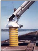
Pivoting gimbal allows different loading angles.
